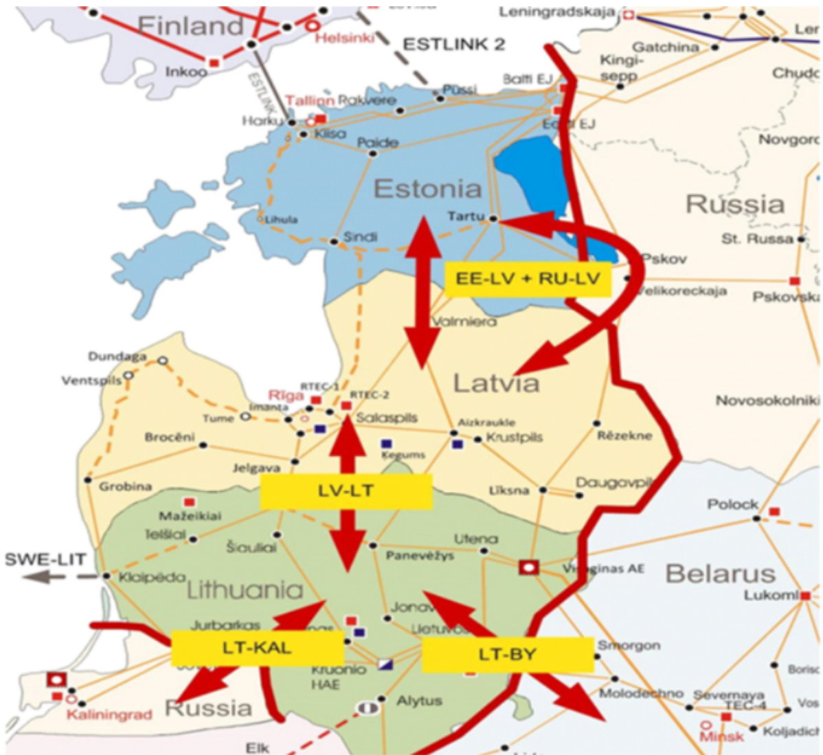
Figure 1: The BRELL power ring. Source: Karčiauskas, 2023.
